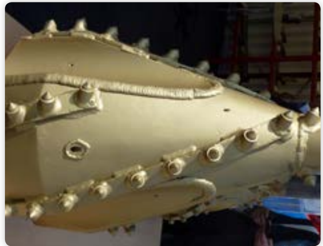
Illustration: HDD reamer with BFZ283
