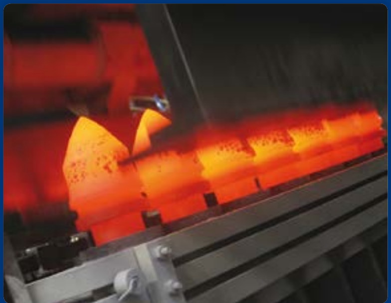
The soldering process to permanently bond tungsten carbide and steel
