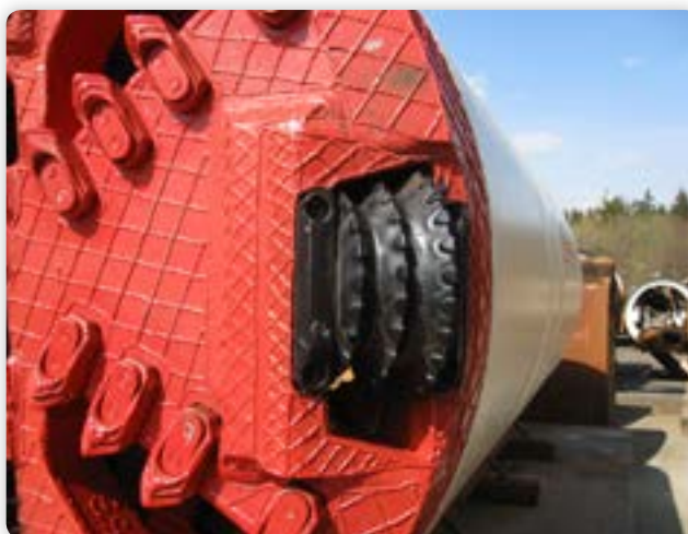
Illustration: Scraper blades BFM70 on a Microtunnelling machine
